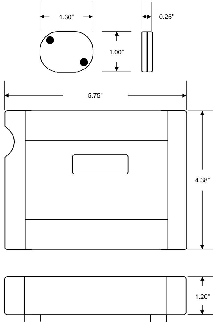
Figure 3. MicroCure and DataReader Case Dimensions
