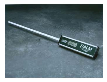
Light Guide to the base of the Probe body where the UV filter passes the UV light of interest to the photodetector. The photodetector converts the light energy to a current that is proportional to its intensity. The signal is conditioned, digitized, processed and displayed on the LCD of the PALM Probe.
