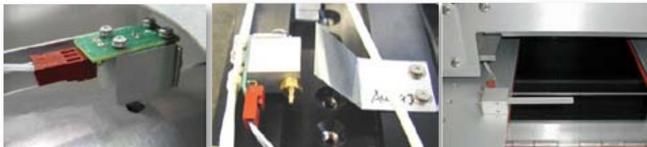
Examples of Compact Sensor Mounting Locations Left to Right: Mounted behind the reflector looking at bulb, mounted behind reflector looking at reflected UV, mounted near cure surface and using quartz rod to pick up UV
