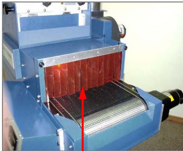
Tunnel Light Curtain
