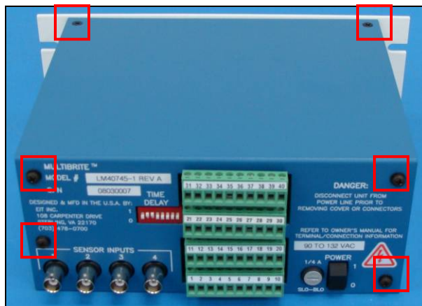
Figure 42: Multibrite® Top and Back Cover Screws
