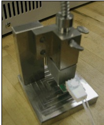
Figure 13: CS-2 Mounted on Fixture with Spot Source Light Guide
