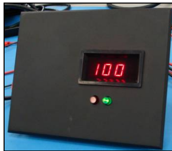
Figure 35: Online UV Intensity Display Module™ 100% UV Intensity
